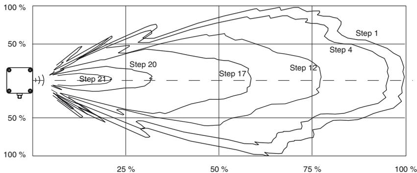
**Sensitivity adjustment for suppression of disturbing targets**
